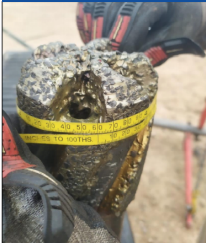
3.61" OD Junk Mill after milling thru 18 plugs.
