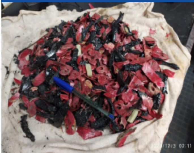
Debris with 3.61" OD mill.
