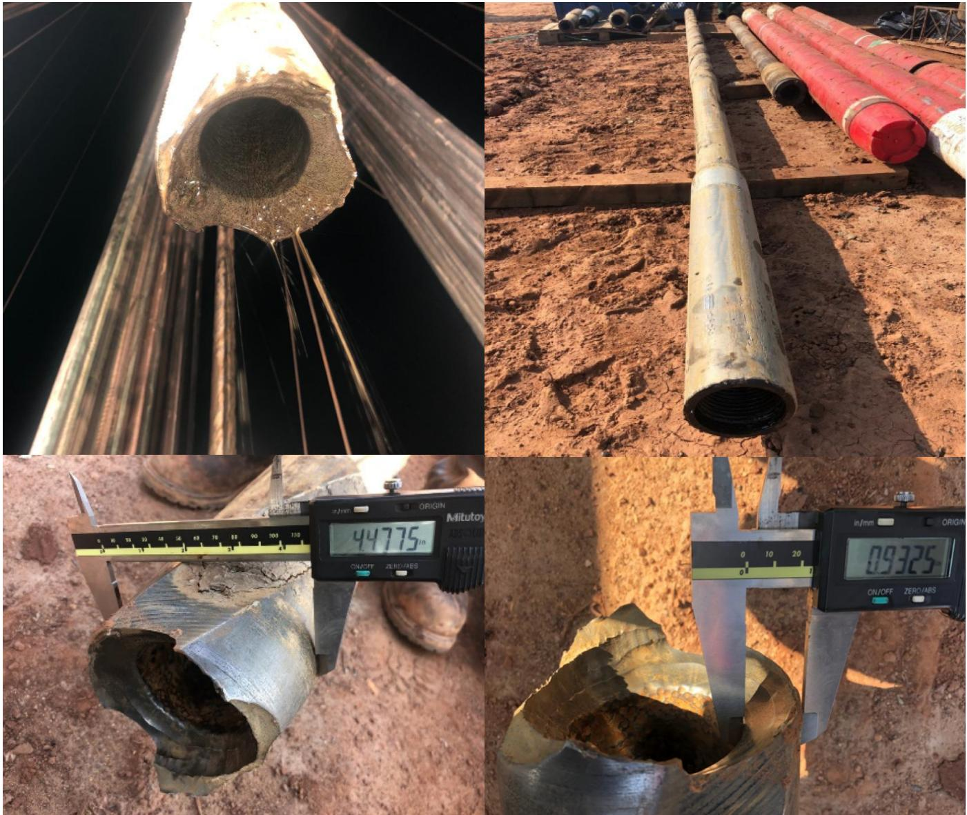
HWDP recovered at surface, showing a clean cut preserving the OD of the string.
